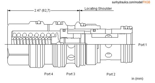
This valve is a 2-way, 2-position proportional throttle. Ports 2 and 3 are normally closed. Pilot pressure at port 1 creates a metering orifice between port 2 and 3 that is proportional to the pressure at 1. The force balance of the flow forces, spring and pilot pressure results in a degree of partial self-compensation as the load pressure changes.
