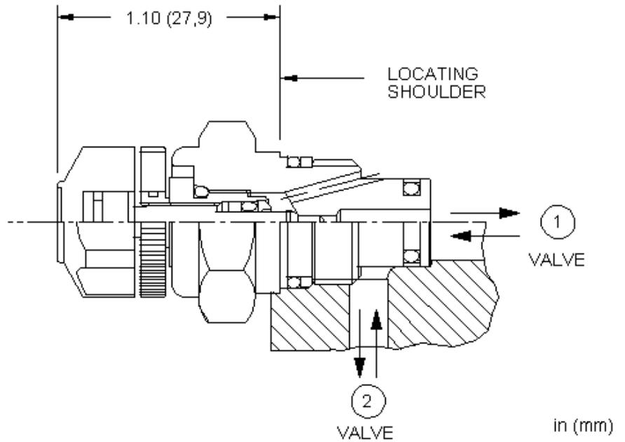
Two-port, pilot-stage needle valves are fully adjustable devices used to regulate pilot flow in a main-stage valve or to meter in/out flow in low flow applications. These cartridges are designed for pilot flow applications and utilize Sun's T-8A cavity so they can be used in conjunction with Sun's pilot-operated, main-stage valves.
