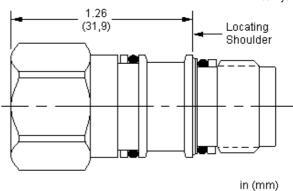
This cavity plug allows ports 1 and 2 to remain open and blocks port 3.
