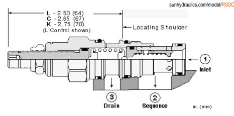
Pilot-operated, balanced piston sequence valves will supply a secondary circuit with flow once the pressure at the inlet (port 1) has exceeded the valve setting. The pressure setting of a sequence valve controls the pressure at port 1 relative to the pressure at the drain (port 3). These valves are insensitive to back pressure at port 2 (sequence), up to the valve setting. They may be used to regulate pressure in place of 2-port relief valves if there is pressure in the return line.
