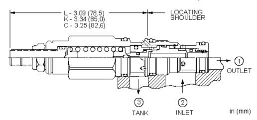
The relief-after-check cartridge is a CavitySaver™ (multi-function) valve incorporating a direct-acting relief tee'd in after a check function. The check valve flow is from the inlet (port 2) to the system port (port1). When the pressure in the system (port 1) reaches the relief valve setting, the valve starts to open to tank (port 3), throttling flow to limit the pressure rise. These valves are smooth and quiet, essentially zero-leak, dirt-tolerant, immune to silting and are very fast.
