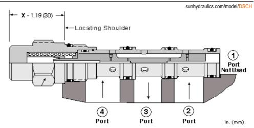
Low-side (hot oil) shuttle cartridges allow hot oil to be diverted from the low pressure side of a closed loop system. When both work ports (ports 2 and 4) are at equal pressures the valve is spring-centered to an all-ports-blocked position. When one of the work ports (port 2 or 4) sees a higher pressure the opposite work port is connected to the common port (port 3).
