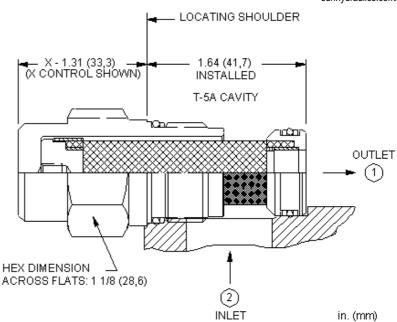
Sun filter elements are available as Surface Type (Last Chance) and Depth Style elements. The flow path is Port 2 to Port 1 and should not be used in reverse, even with a reverse free flow check valve installed. The elements have a high collapse pressure and are intended to be used in line with the system. Filter life will depend on initial system cleanliness and the amount of dirt ingression to the system when operating.
