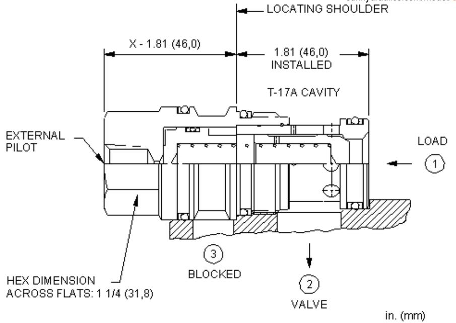
This valve is a spring biased closed, pilot-to-close check cartridge that has a 1.8:1 pilot ratio. The valve allows flow from port 1 to port 2 and blocks reverse flow. Pressure at the external pilot port opposes pressure at port 1 at a ratio of 1.8:1. Port 3 is blocked.
