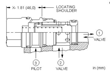
These unbalanced, pilot-to-close logic valves are 2-way switching elements that are spring biased closed. Pressure at either work port 1 or 2 will oppose the spring and tend to open the valve while pressure at port 3 will tend to close it. The force generated at port 3, plus the spring force, must be greater than the sum of the forces acting at port 1 and port 2 for the valve to remain closed. NOTE: The pilot area (port 3) is 1.8 times the area at port 1 and 2.25 times the area at port 2.
