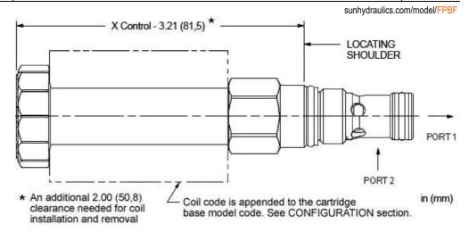
This valve is a pilot-operated, normally closed, electro-proportional throttle with reverse free-flow check. Energizing the coil generates an opening force on the pilot stage which vents the main stage poppet to open proportionally, allowing flow from port 2 to 1. In the open condition, flow from 1 to 2 will cause the valve to auto-close and only pilot flow will pass from 1 to 2.
