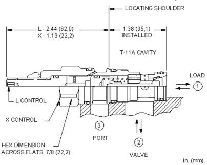
This valve is a pilot to open check valve. It has a sealed pilot, a Delrin seat, and is non-vented. It allows free flow from the valve (port 2) to the load (port 1) and blocks flow in the opposite direction. Pressure at the pilot (port 3) will open the valve from port 1 to port 2. Pilot pressure needed at port 3 to open the valve is directly proportional to the load pressure at port 1. Pressure at port 2 directly opposes pilot pressure.
