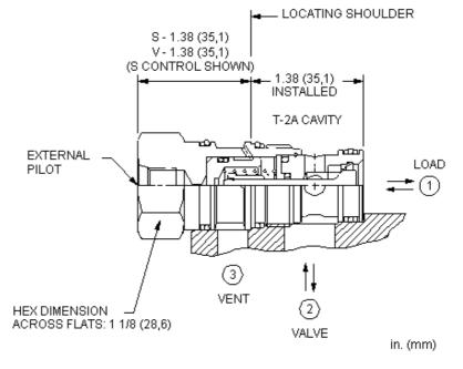
This valve is a pilot to open check valve. It has a sealed pilot, a Delrin seat, and is vented. It allows free flow from the valve (port 2) to the load (port 1) and blocks flow in the opposite direction. Pressure at the external pilot port will open the valve from port 1 to port 2. Pilot pressure needed to open the valve is directly proportional to the load pressure at port 1. The valve is insensitive to pressure at port 2 because the spring chamber references the vent (port 3).
