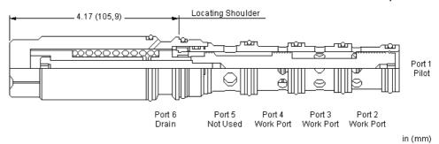
Two-position, 3-way directional cartridges are 6-port (port 5 is not used) directional valves that can be configured with up to 5 different spool configurations. The supply port is port 3 and all ports will accept 5000 psi (350 bar). Capacity for these pilot-to-shift valves is dependent on the spool type specified.
