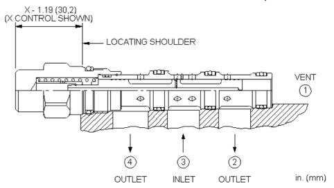
This is a vent-to-shift, 2-position, diverter valve that is normally closed. When port 1 is vented, the pressure differential between port 3 and port 1 exceeds the spring force causing the valve to shift, thereby connecting port 3 with ports 2 and 4.
