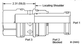
This cavity plug allows ports 1 and 3 to remain open and blocks port 2.
