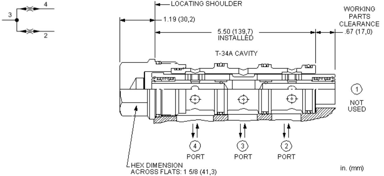
High accuracy, closed-center flow divider/combiners are sliding-spool, pressure-compensated devices used to split flow in one direction and combine flow in the opposite direction. These valves may be used to accurately control two or more cylinders or hydraulic motors where bidirectional operation is required.
