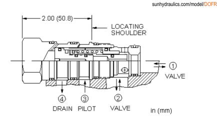
This is a normally open, balanced poppet, switching element. When the vent port (port 4) is blocked, the poppet remains in the open position. Venting port 4 shifts it to the closed position, provided there is sufficient pressure at port 3.
