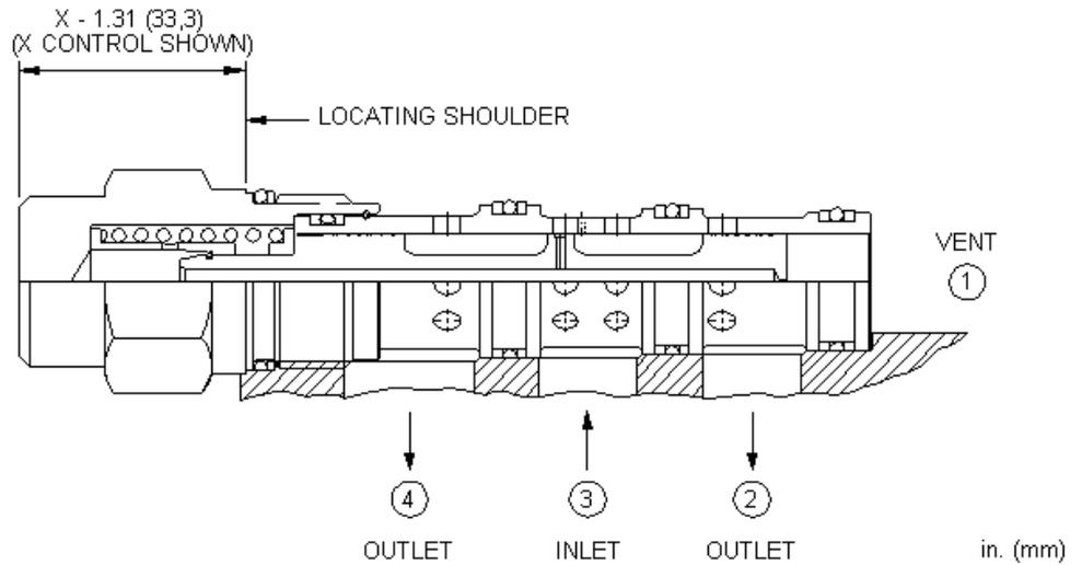
This is a vent-to-shift, 2-position, diverter valve that is normally closed. When port 1 is vented, the pressure differential between port 3 and port 1 exceeds the spring force causing the valve to shift, thereby connecting port 3 with ports 2 and 4.
