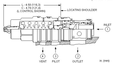
Vented counterbalance valves with pilot assist are meant to control an overrunning load. The check valve allows free flow from the directional valve (port 2) to the load (port 1) while a direct-acting, pilot-assisted relief valve controls flow from port 1 to port 2. Pilot assist at port 3 lowers the effective setting of the relief valve at a rate determined by the pilot ratio. Backpressure at port 2 does not affect the valve setting because the spring chamber references the vent (port 4).
