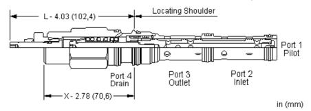
This valve is a 2-way, 2-position proportional throttle. Ports 2 and 3 are normally closed. Pilot pressure at port 1 opposes the spring and creates a variable metering orifice between port 2 and 3 that is proportional to the pressure at 1. The force balance of the flow forces, spring and pilot pressure results in a degree of partial self-compensation as the load pressure changes.
