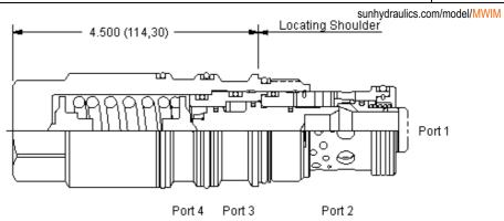
Vented, balanced load control valves combine a balanced modulating element with a reverse flow check. The check valve allows free flow from the directional valve (port 2) to the load (port 1) while the pilot to open modulating element controls flow from port 1 to port 2. Pilot pressure at port 3 determines the flow setting. Backpressure at port 2 does not affect the flow setting because the spring chamber references the vent (port 4).
