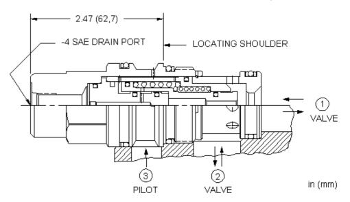
This is a normally open, balanced poppet, switching element. When the external vent port is blocked, the poppet remains in the open position. Venting the external port shifts it to the closed position, provided there is sufficient pressure at port 3.
