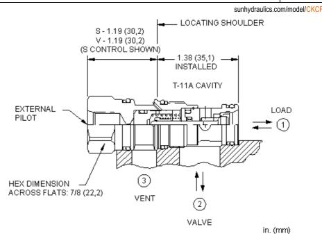
This valve is a pilot to open check valve. It has a sealed pilot, a steel seat, and is vented. It allows free flow from the valve (port 2) to the load (port 1) and blocks flow in the opposite direction. Pressure at the external pilot port will open the valve from port 1 to port 2. Pilot pressure needed to open the valve is directly proportional to the load pressure at port 1. The valve is insensitive to pressure at port 2 because the spring chamber references the vent (port 3).
