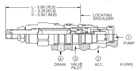
The accumulator sense, pump unload pilot valve is used to sense pressure in an accumulator at port 2 of the valve and when the pressure at port 2 reaches the valve setting, port 3 connects to port 4 to vent a relief valve and unload the pump. This valve has a 20% ratio between unload setting and reset; when pressure at port 2 falls below 80% of the valve setting, port 3 is blocked from port 4 and the pump will come back online to recharge the accumulator.
