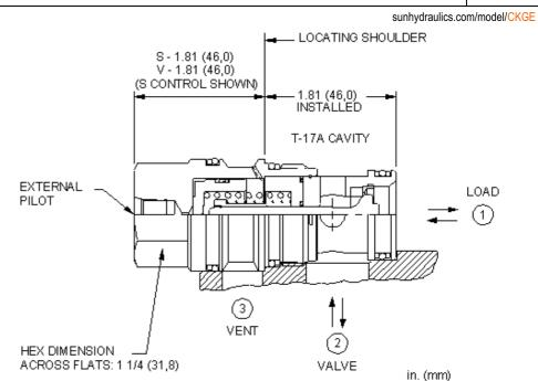
This valve is a pilot to open check valve. It has a sealed pilot, a Delrin seat, and is vented. It allows free flow from the valve (port 2) to the load (port 1) and blocks flow in the opposite direction. Pressure at the external pilot port will open the valve from port 1 to port 2. Pilot pressure needed to open the valve is directly proportional to the load pressure at port 1. The valve is insensitive to pressure at port 2 because the spring chamber references the vent (port 3).
