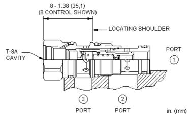
This valve is a, 3-way directional cartridge (1 blocked, 2 to 3 open) that incorporates an integral pilot control cavity. It may be used by itself or to actuate larger pilot-operated directional cartridges or logic elements. The valve shifts when there is flow through the pilot control cartridge installed in the T-8A cavity.
