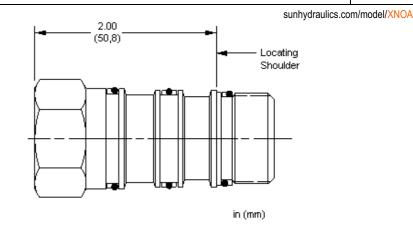
These cavity plugs can be used for both four-port and six-port cavities. When used in four-port cavities (T-21A, T-22A, T-23A and T-24A), ports 1 and 2 remain connected and ports 3 and 4 are blocked. When used in six-port cavities (T-61A, T-62A, T-63A and T-64A), ports 1, 2, 3 and 4 remain connected and ports 5 and 6 are blocked.
