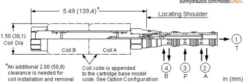
This direct acting, solenoid-operated, 4-way, 3-position spool valve is spring centered to the neutral position. When coil A is energized, the flow is from port 3 (P) to port 2 (A) and from port 4 (B) to port 1 (T). When coil B is energized, the flow is from port 3 to port 4 and from port 2 to port 1.
