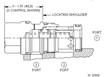
Normally closed modulating elements without an internal orifice act as a bypass compensator to maintain a constant pressure drop across an orifice, regardless of variations in upstream or downstream pressure.
