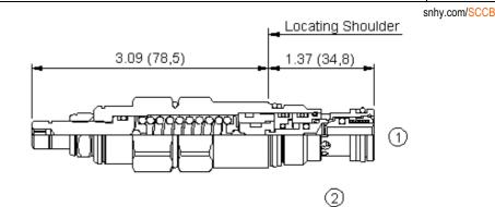
Atmospherically referenced, direct-acting sequence valves with reverse-flow check will supply a secondary circuit with flow once the pressure at the inlet (port 1) has exceeded the valve setting. Additionally, these valves incorporate an integral check valve to provide reverse flow from port 2 (sequence) to port 1 (inlet). The pressure setting of this sequence valve controls the pressure at port 1 relative to the atmospheric vent.
