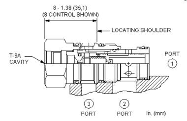
This valve is a normally open, 2-way directional cartridge that incorporates an integral pilot control cavity. It may be used by itself or to actuate larger pilot-operated directional cartridges or logic elements. The valve shifts when there is flow through the pilot control cartridge installed in the T-8A cavity.
