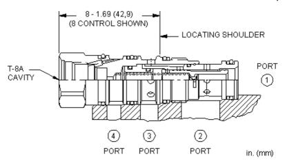
This valve is a, 3-way directional cartridge (1 to 2 open, 3 blocked) that incorporates an integral pilot control cavity. It may be used by itself or to actuate larger pilot-operated directional cartridges or logic elements. The valve shifts when there is flow through the pilot control cartridge installed in the T-8A cavity.
