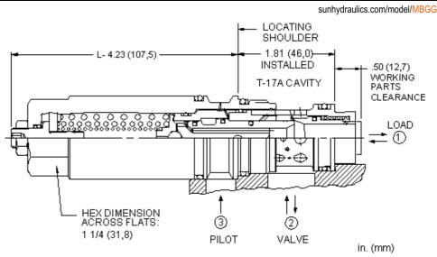
Load reactive, load control valves with pilot assist combine two valves; a check valve and a relief valve. The check valve allows free flow from the directional valve (port 2) to the load (port 1) while a direct-acting, pilot-assisted relief valve controls flow from port 1 to port 2. Pilot assist at port 3 lowers the effective setting of the relief valve at a rate determined by the pilot ratio.
