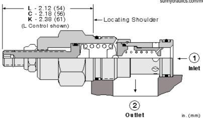
Kick-down relief cartridges act similar to a circuit breaker in an electrical system. The valves will kick completely open and remain open once the pressure at the inlet (port 1) exceeds the valve settling, creating an unrestricted flow path from port 1 to tank (port 2). The valve remains open as long as the pressure at port 1 exceeds the pressure at port 2. To reset the valve, flow from port 1 to port 2 must cease and pressure at port 2 must be equal to or greater than the pressure at port 1.
