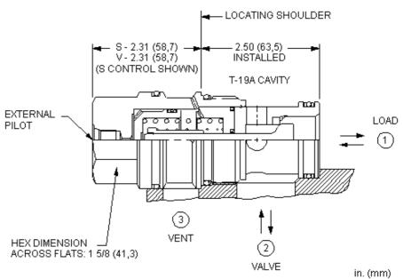
This valve is a pilot to open check valve. It has a sealed pilot, a steel seat, and is vented. It allows free flow from the valve (port 2) to the load (port 1) and blocks flow in the opposite direction. Pressure at the external pilot port will open the valve from port 1 to port 2. Pilot pressure needed to open the valve is directly proportional to the load pressure at port 1. The valve is insensitive to pressure at port 2 because the spring chamber references the vent (port 3).
