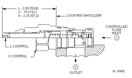
Fixed-orifice, pressure-compensated flow controls provide precise flow regulation for meter-in or meter-out applications where there may be wide pressure fluctuations. The flow setting is specified by the user and is set at the factory.
