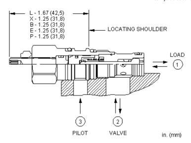
This valve is a pilot to open check valve. It has a non-sealed pilot, a steel seat, and is non-vented. It allows free flow from the valve (port 2) to the load (port 1) and blocks flow in the opposite direction. Pressure at the pilot (port 3) will open the valve from port 1 to port 2. Pilot pressure needed at port 3 to open the valve is directly proportional to the load pressure at port 1. Pressure at port 2 directly opposes pilot pressure.
