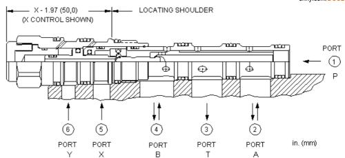
Two-position, detented, 4-way directional cartridges are 6-port directional valves that can be configured with up to 3 different spool options. The supply port is port 1 and all ports will accept 5000 psi (350 bar). Capacity for these pilot-to-shift valves is dependent on the spool type specified.
