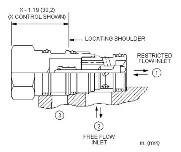
Free-flow, side-to-nose cheater check valves with a bypass orifice function as a 2-port check valve in a 3-port cavity. They allow free flow from port 2 to port 1 with a customer specified orifice that controls flow from port 1 to port 2. Port 3 of the cartridge is blocked off.
