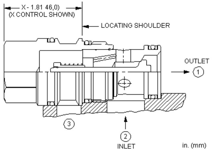
Free-flow, side-to-nose cheater check valves function as a standard 2-port check valve in a 3-port cavity with port 3 of the cartridge blocked off. These valves are useful in circuits where a check valve is required in an existing three port cavity.
