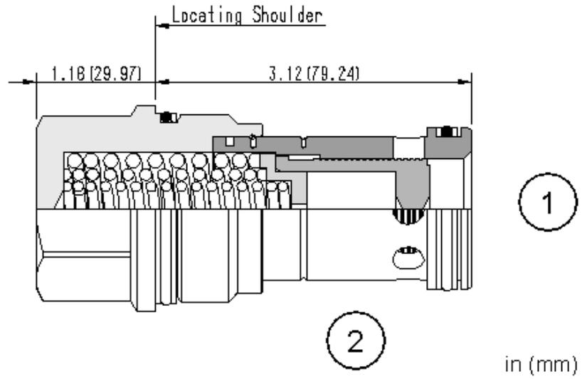
This valve was designed to be used in a parts-in-body, hot oil shuttle assembly. 2 valves, nose to nose, with a pin in between created the low side shuttle.
