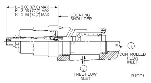
Needle valves with reverse-flow check are fully adjustable orifices used to regulate flow. They are infinitely adjustable from fully closed up to the maximum orifice diameter. An integral high-capacity check valve provides unrestricted flow from port 2 to port 1. They are not pressure compensated.
