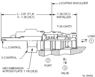
This valve is a pilot to open check valve. It has a sealed pilot, a steel seat, and is non-vented. It allows free flow from the valve (port 2) to the load (port 1) and blocks flow in the opposite direction. Pressure at the pilot (port 3) will open the valve from port 1 to port 2. Pilot pressure needed at port 3 to open the valve is directly proportional to the load pressure at port 1. Pressure at port 2 directly opposes pilot pressure.
