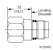
These cavity plugs can be used for both two-port and four-port cavities and allow all ports to remain connected.
