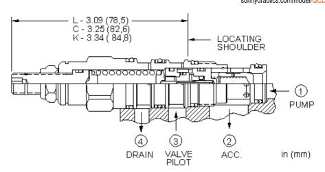
The accumulator sense, pump unload pilot valve is used to sense pressure in an accumulator at port 2 of the valve and when the pressure at port 2 reaches the valve setting, port 3 connects to port 4 to vent a relief valve and unload the pump. This valve has a 50% ratio between unload setting and reset; when pressure at port 2 falls below 50% of the valve setting, port 3 is blocked from port 4 and the pump will come back online to recharge the accumulator.
