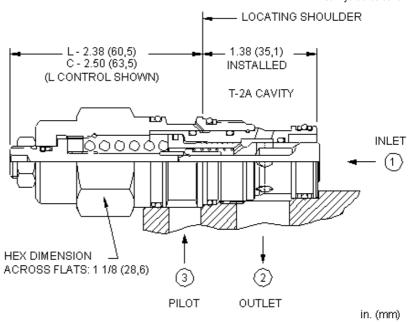
Counterbalance valves with pilot assist are meant to control an overrunning load. The check valve allows free flow from the directional valve (port 2) to the load (port 1) while a direct-acting, pilot-assisted relief valve controls flow from port 1 to port 2. Pilot assist at port 3 lowers the effective setting of the relief valve at a rate determined by the pilot ratio.
