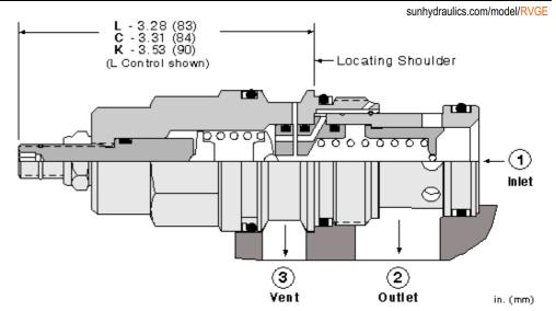
Fast-acting, ventable, pilot-operated, balanced piston relief cartridges are normally closed pressure regulating valves. When the pressure at the inlet (port 1) reaches the valve setting, the valve starts to open to tank (port 2), throttling flow to regulate the pressure. They provide a vent port (port 3) that connects between the main piston and pilot stage to provide for remote control by other pilot or 2-way valves. These valves have low pressure rise vs. flow and are very fast.
