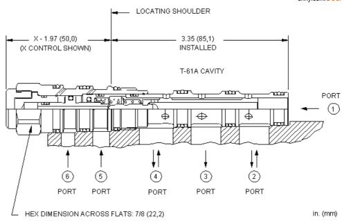
Three-position, 4-way directional cartridges are spring-centered, 6-port directional valves that can be configured from a choice of 10 different spool options. The supply port is port 1 and all ports will accept 5000 psi (350 bar). Capacity for these pilot-to-shift valves is dependent on the spool type specified.
