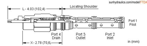
This valve is a 2-way, 2-position proportional throttle. Ports 2 and 3 are normally closed. Pilot pressure at port 1 opposes the spring and creates a variable metering orifice between port 2 and 3 that is proportional to the pressure at 1. The force balance of the flow forces, spring and pilot pressure results in a degree of partial self-compensation as the load pressure changes.
