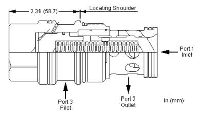
This valve is a spring biased closed, pilot-to-close check cartridge that has a 1.8:1 pilot ratio. The valve allows flow from port 1 to port 2 and blocks reverse flow. Pressure at the pilot port opposes pressure at port 1 at a ratio of 1.8:1. This valve is most often used in regeneration circuits.
